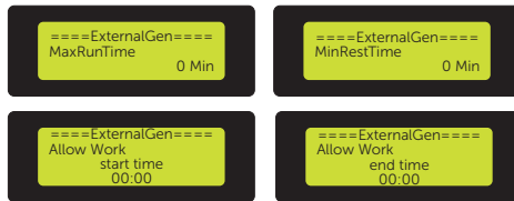
Figure 9-79 Setting MaxRunTime, MinRestTime, allow working period
