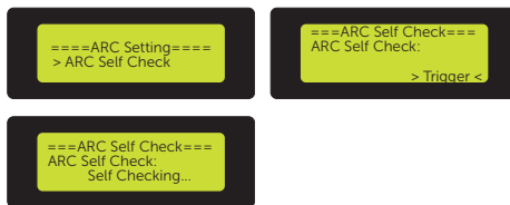
Figure 9-101 Triggering ARC Self Check
